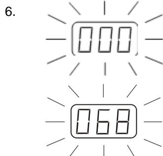
If **000** flashes on the display, a reset is necessary. This procedure is explained in section 4.2.4.
