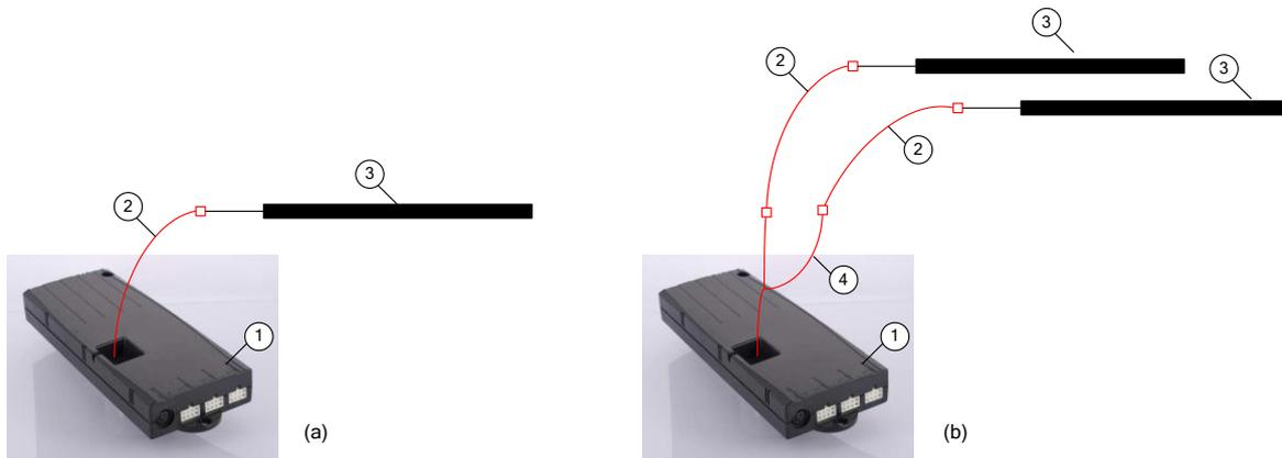
Figure 6: connection of (a) one squeeze line and (b) two squeeze lines
