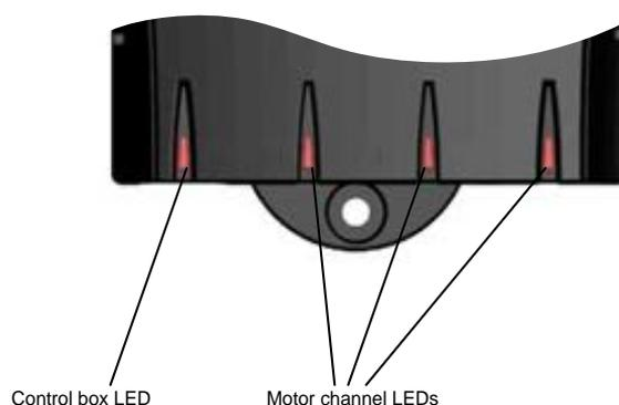
Figure 7: LEDs on COMPACT<sup>eco</sup>
